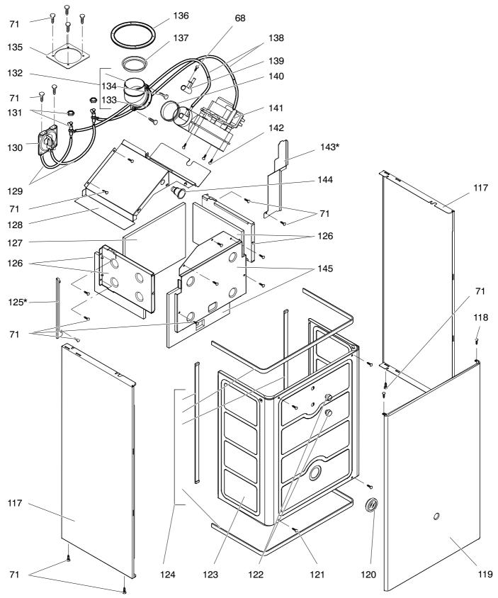
Fan, combustion chamber and case panels
